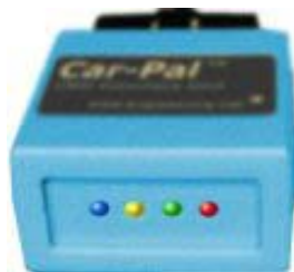
Figure 3 – Status LED's at the Rear of the Car-Pal™ OBD Interface Unit.
